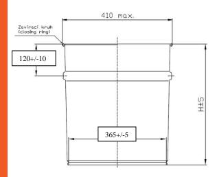
32 l: H = 330 ±5 mm 45 l: H = 420 ±5 mm 55 l: H = 530 ±5 mm 60 l: H = 590 ±5 mm 65 l: H = 630 ±5 mm
